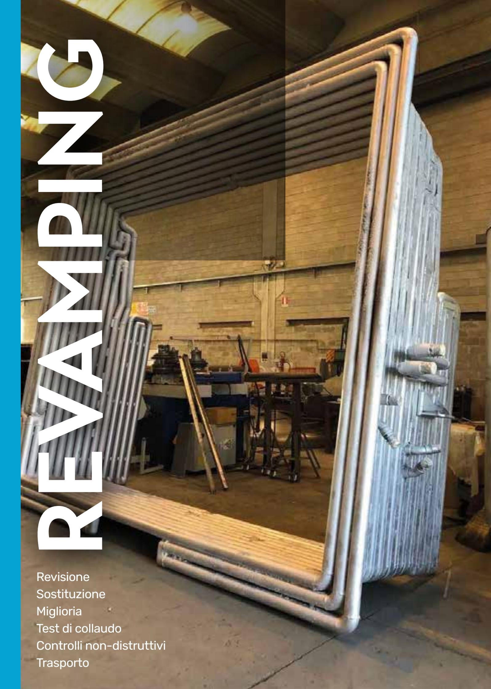
A large industrial heat exchanger, possibly a condenser or evaporator, is shown in a factory setting. The unit is composed of numerous parallel tubes bundled together in a rectangular frame. It is positioned on a concrete floor, and various tools and equipment are visible in the background, including a workbench and a ladder. The lighting is industrial, with overhead fixtures illuminating the scene.
